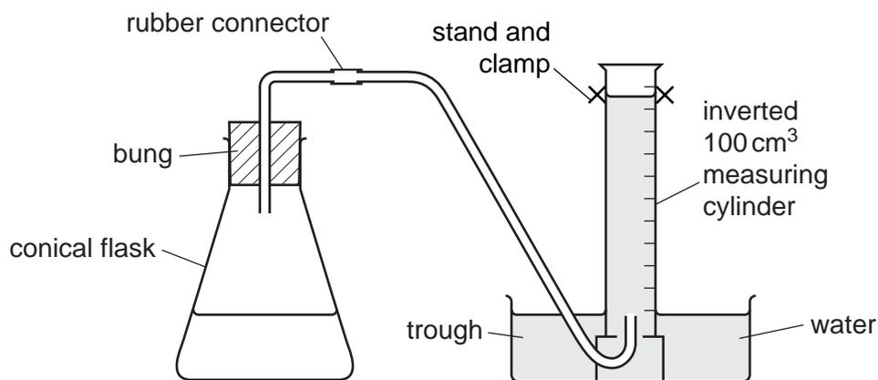
Using a measuring cylinder,  $50\text{ cm}^3$  of dilute acid **X** was poured into the conical flask.  $0.5\text{ g}$  of magnesium ribbon was added to the conical flask and the bung added.
